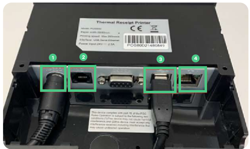
Figure 2. Printer with port for Power, Cash Drawer (Labelled DK) and USB Connection to POS Bridge Station.
